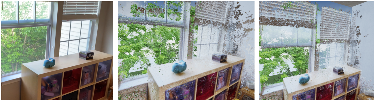
Figure 5.1: Left : ground truth image. Before ( Middle ) and after ( Right ) audio-augmented rendering of an indoor scene with open and closed reflective surfaces. The reconstruction is enhanced by EchoCNN inferences of surface detection, depth estimation, and material classification based on audio-visual reflecting sound and image inputs.
